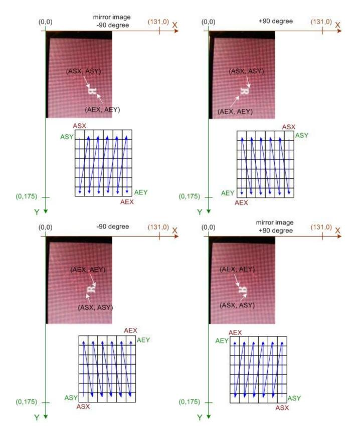
The given programming sequences are using the definition of the picture writing routine above. Note that the width (CHAR\_W) and the height (CHAR\_H) have to be swapped, if the image is displayed in a 90 degree rotation. Inital, before starting data writing and address mode changing, the register have to be defined and the addressing mode has to be set using the following code sequence:
